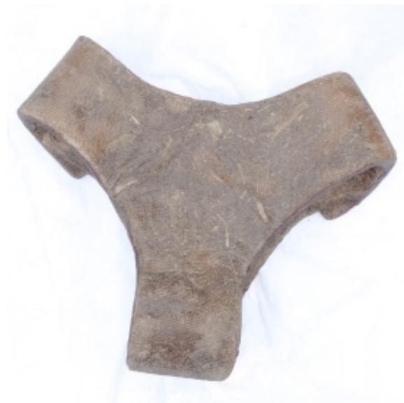
the first iteration of the fullscale prototype turned out heavier than expected and needed a suport structure that relies on compression to keep the legs from opening and the seat from sinking lower
