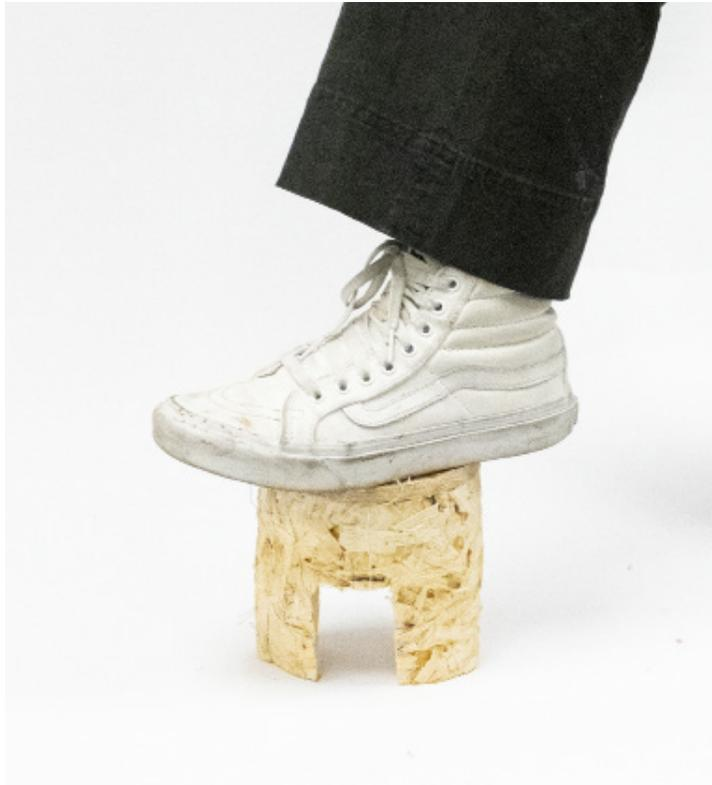
1/4 scale prototype made from compressed corn husks and 20% beeswax and 80% pine resin in the shape of a semi column held under 60 kilos.
