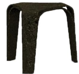
to avoid making a second mould for the cross brace and to give the piece more structural support I decided to laminate two thinner pieces.
