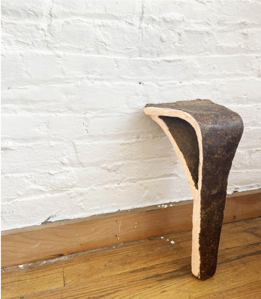
I decided to focus on a full scale sample of the leg because of constant rain that delayed the drying process. the sample turned out to be considerably lighter than the previous and was able to support 50lbs.
