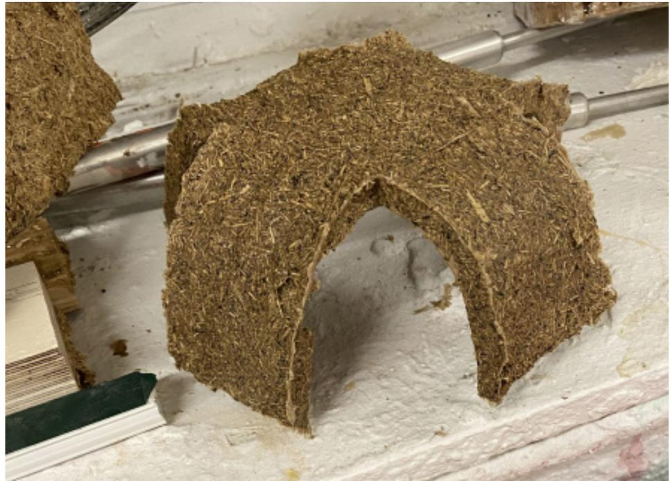
bent 1/4 scale model hide glue and ground corn husks
